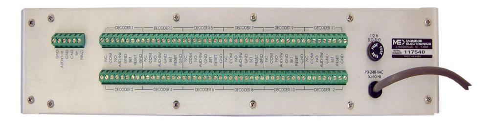
The terminal blocks are in groups of 8 inputs, with each group associated with one of the 3185E cards installed. NC is the normally closed contact on the 3185E board, NO the normally open contact, and the COM terminal s the common of the relay contacts.
